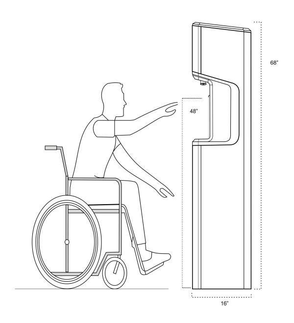
ADA Reach Compliance: Where a forward reach is unobstructed, the high forward reach shall be 48 inches (1220 mm) maximum and the low forward reach shall be 15 inches (380 mm) minimum above the finish floor or ground.
