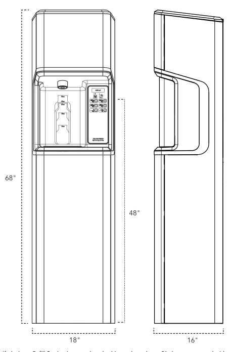
Note: If placing a Refill Station in an enclosed cabinet, please leave 3" clearance on each side, and 6" clearance to the rear. Ensure that there is sufficient venting.
